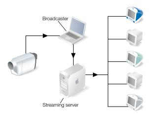
A PowerBook G4 with QuickTime Broadcaster software captures and encodes video and audio. The encoded signal is sent over an Internet Protocol (IP) network to a server computer running QTSS or DSS software. QTSS or DSS on the server computer sends the signal over the Internet or a local network to client computers that tune in using QuickTime Player.
